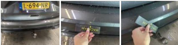
Bumper R, Scratch(es), Repair and paint (complete)
