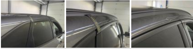
Door FR, Dent(s), Repair and paint (complete)
