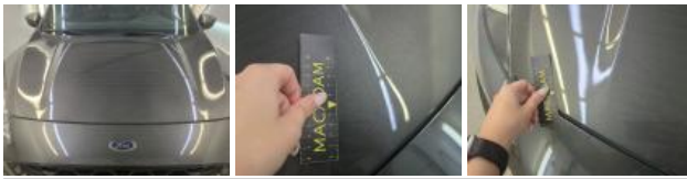
Roof pillar R, Dent(s), Paintless dent repair
