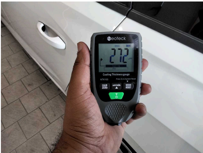
Side panel - rear left side: 272 \mu\text{m}
