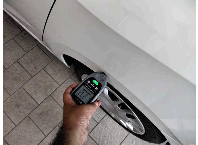
Side panel - rear left side: 272 \mu\text{m}
