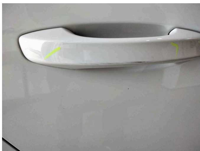
Damage 1: Door - rear right side: Door handle - outside - Scratch(es) - Smart repair
