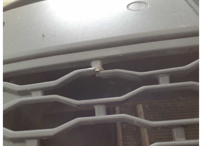
Damage 5: Front bumper: Front bumper - Damaged - Replace
