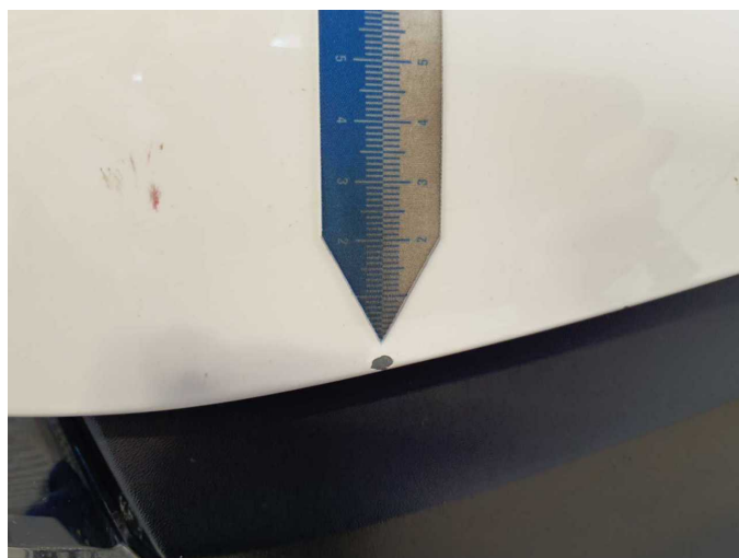
Damage 6: Bonnet: Bonnet - Corrosion - Paint
