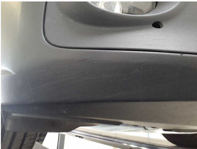
Damage 5: Front bumper: Front bumper - Damaged - Replace
