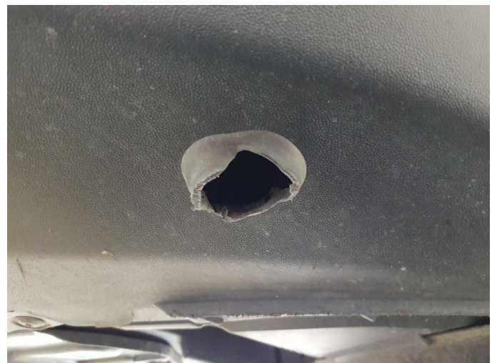
Damage 5: Front bumper: Front bumper - Damaged - Replace
