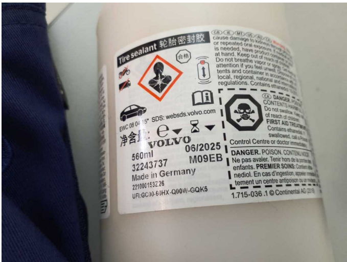
Damage 1: Equipment: Tirefit filler - Expired - Replace
