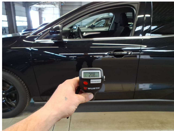
Repainting 1: Door - front left side
