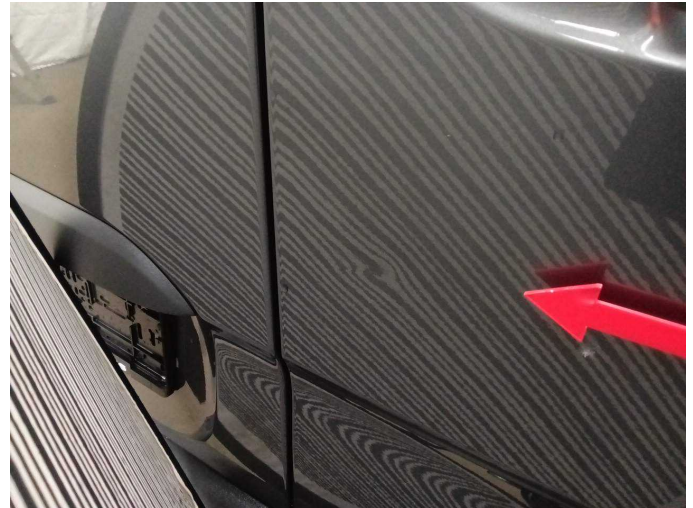
Damage 8: Boot lid / rear door: Rear door - right side - Dent / paintcoat damage - Smart repair
