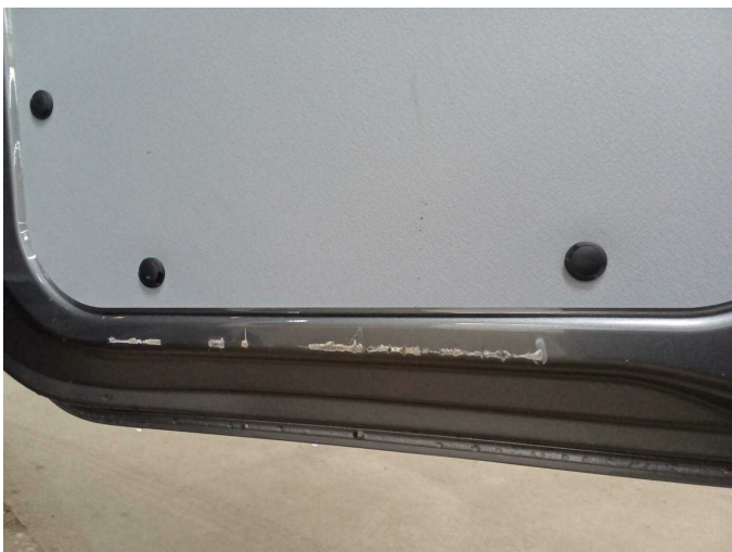
Damage 10: Boot lid / rear door: Rear door - right side (innen) - Dent / paintcoat damage - Smart repair
