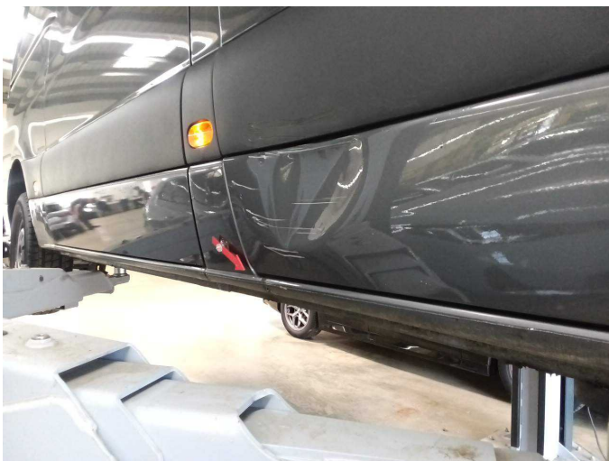
Damage 7: Sill - right side: Sill - Scratched - Smart repair
