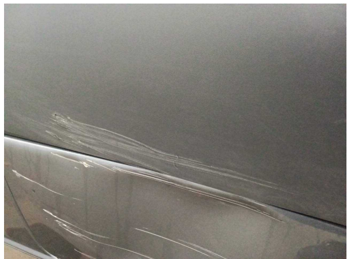
Damage 5: Door - front right side: Brightware - lower - Scratched - Replace
