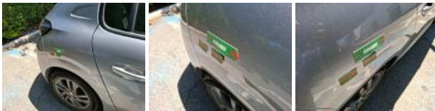
Door RR, Dent(s), Repair and paint (complete)
