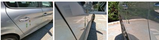
Door FR, Dent(s), Repair and paint (complete)
