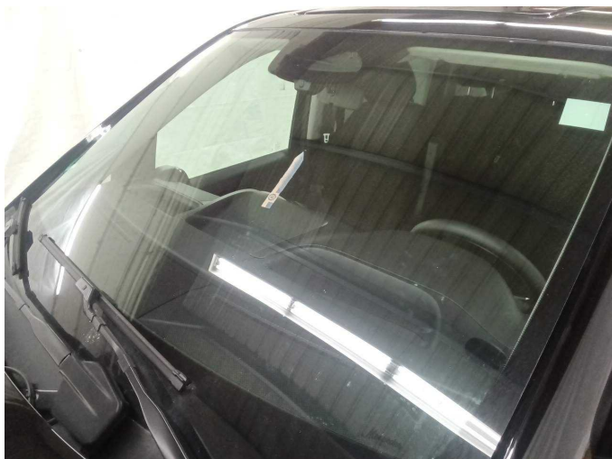
Damage 10: Vehicle glazing: Windscreen - Stone chips - Replace
