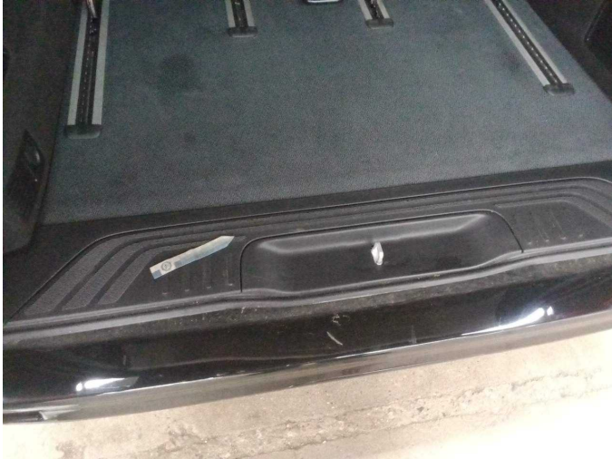
Damage 3: Trim / covers: Boot sill cover - Scratched - Loss in value
