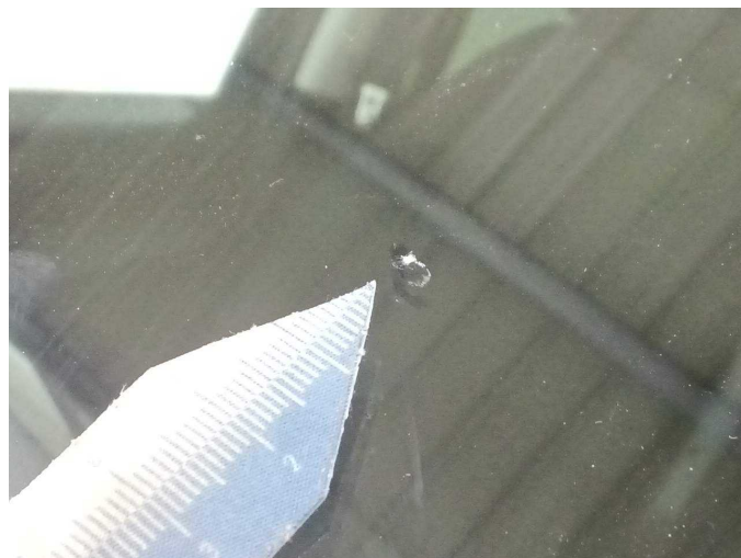
Damage 10: Vehicle glazing: Windscreen - Stone chips - Replace
