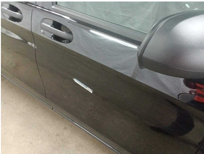
Damage 7: Door - front right side: Door - dent(s) - Smooth repair work
