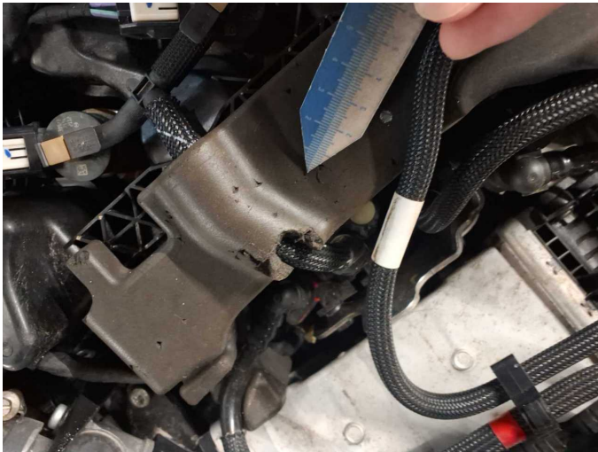
Damage 1: Misc.: Misc. (Isolierung Motor) - Damage caused by marten / rodent - Replace
