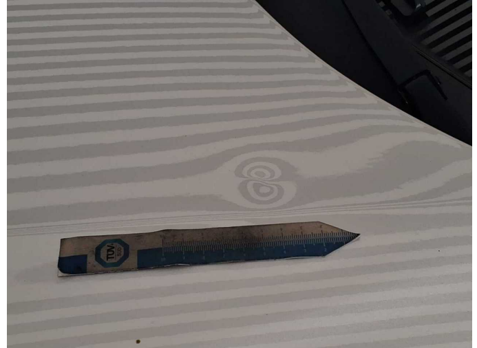
Damage 4: Bonnet: Bonnet - dent(s) - Smooth repair work
