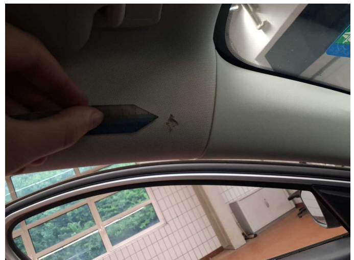
Damage 10: Trim / covers: Roof lining - Burn hole (cigarettes) - Replace
