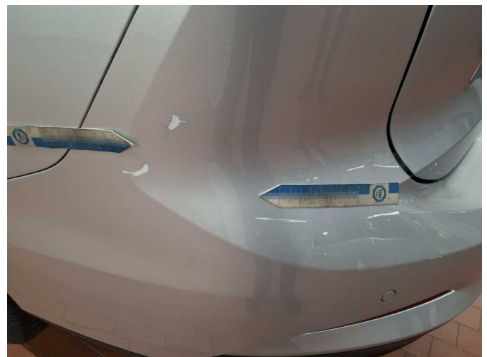
Damage 6: Rear bumper: Rear bumper - Scratched - Paint
