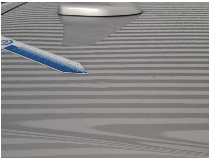
Damage 3: Roof: Roof - dent(s) - Smooth repair work
