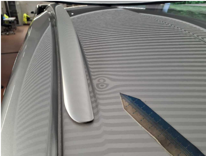
Damage 3: Roof: Roof - dent(s) - Smooth repair work
