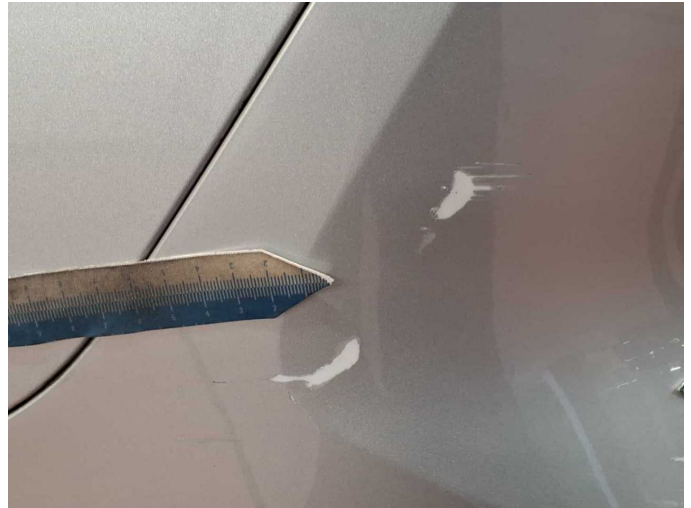
Damage 6: Rear bumper: Rear bumper - Scratched - Paint
