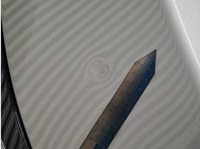
Damage 4: Bonnet: Bonnet - dent(s) - Smooth repair work
