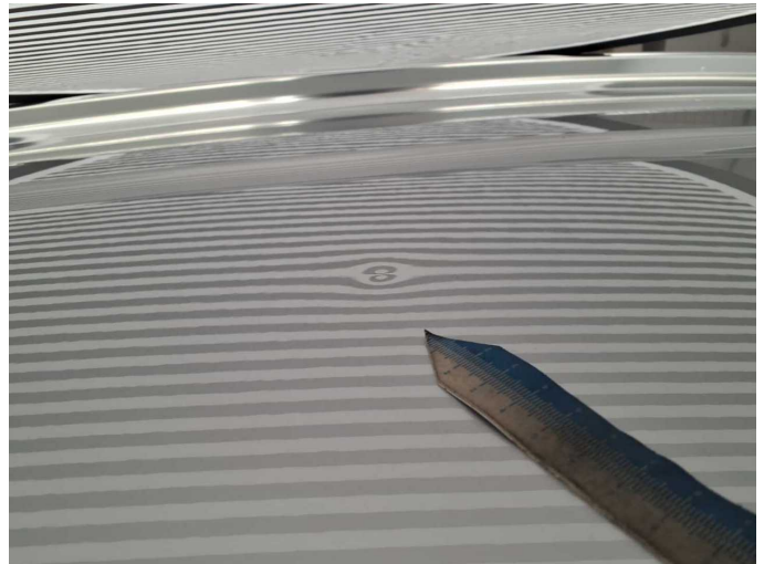
Damage 3: Roof: Roof - dent(s) - Smooth repair work
