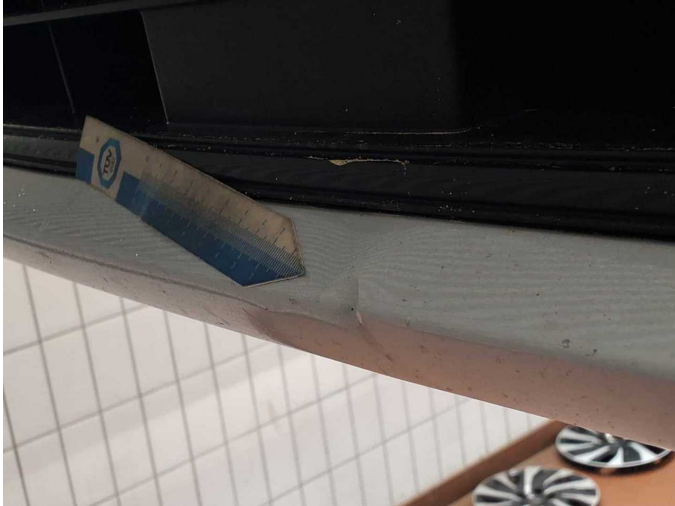
Damage 7: Front bumper: Front bumper (+ Steinschläge) - Dent / paintcoat damage - Repair and paint
