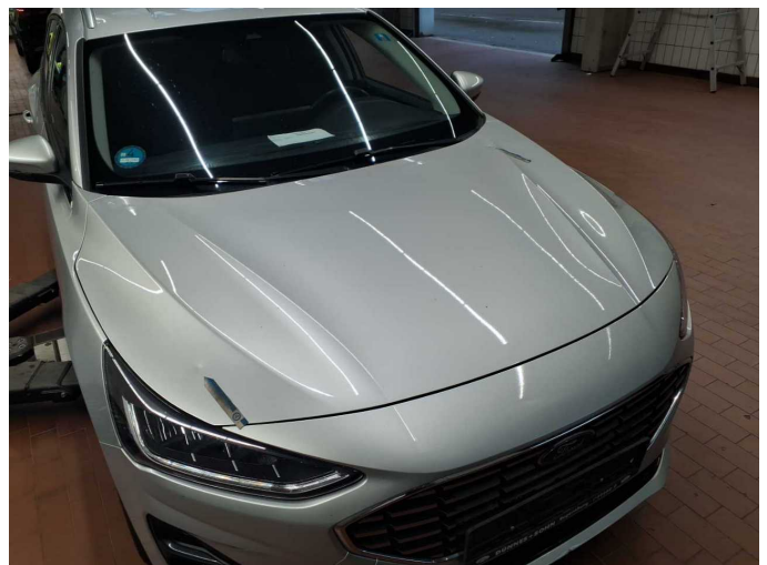
Damage 4: Bonnet: Bonnet - dent(s) - Smooth repair work
