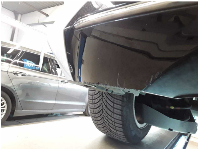
Damage 4: Rear bumper: Rear bumper (unterhalb) - Scratched - Smart repair
