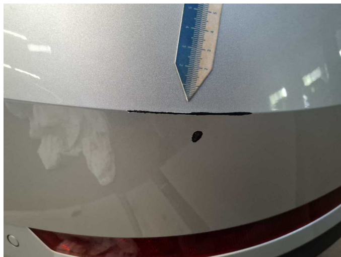
Damage 6: Rear bumper: Rear bumper - Scratched - Paint
