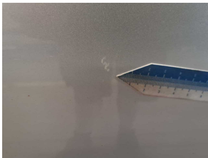
Damage 5: Door - front right side: Door - Scratched - Smart repair
