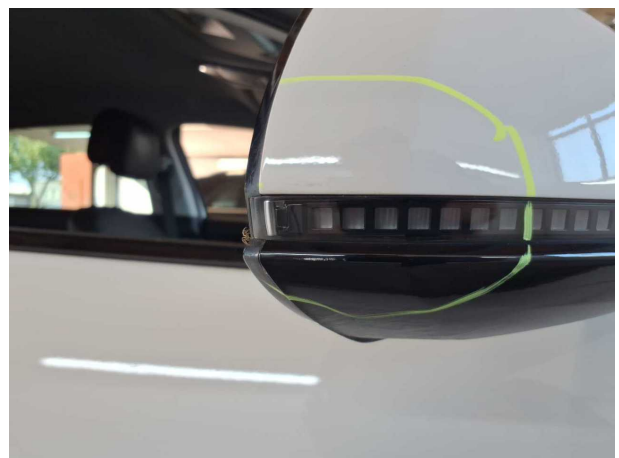
Damage #4: Wing mirror - right side: Mirror housing - Scratch... - Smart repair
