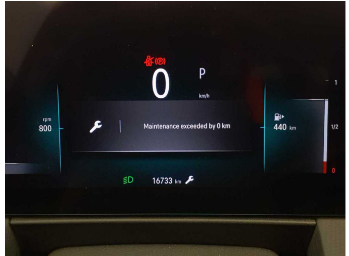
Damage 3: Misc.: Inspection / maintenance - Due - Replace
