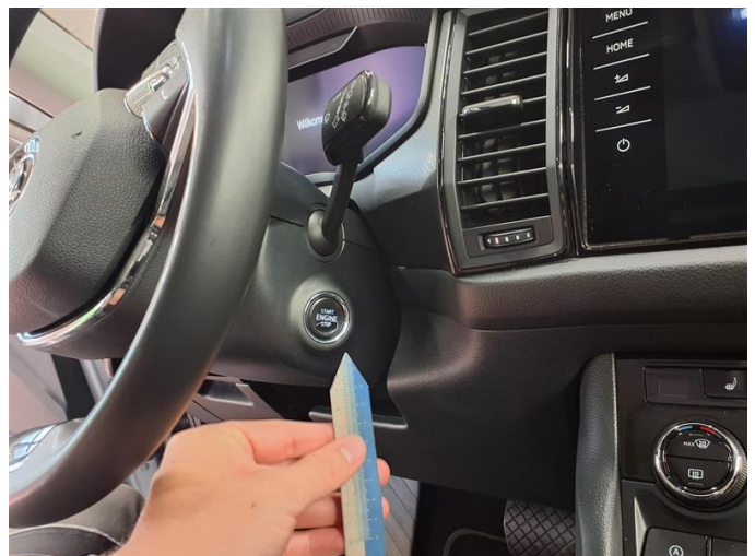
Damage 1: Instrument panel: Cover (Startknopf) - Broken / torn - Replace
