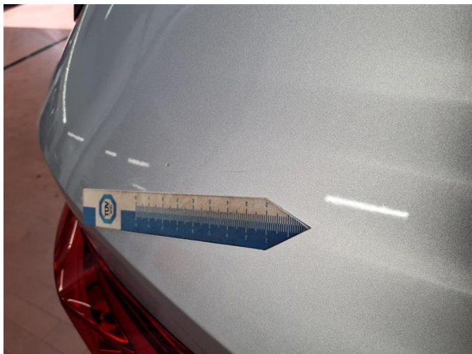
Wear and tear 5: Side panel - rear right side: Side panel - Scratch(es) - Conditioning
