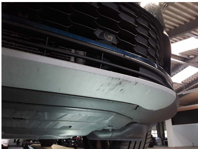
Damage 5: Front bumper: Spoiler - Scratch(es) - Smart repair
