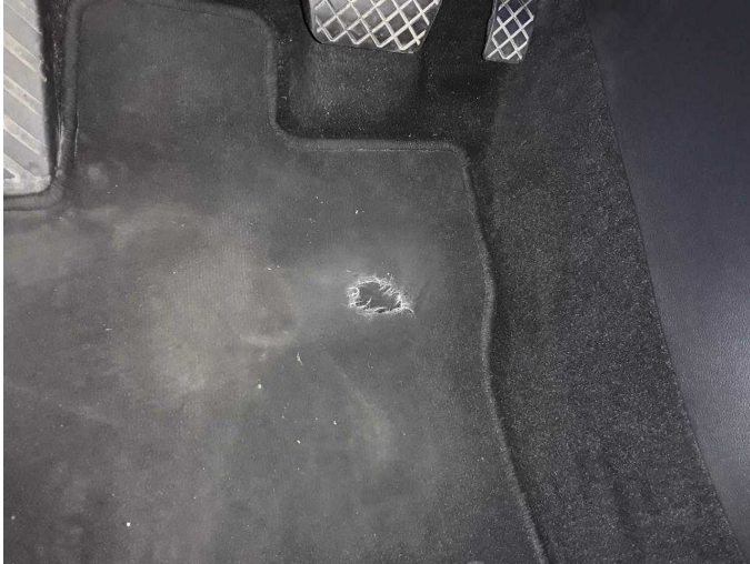
Wear and tear 9: Trim / covers: Floor mats - Broken / torn - No deduction
