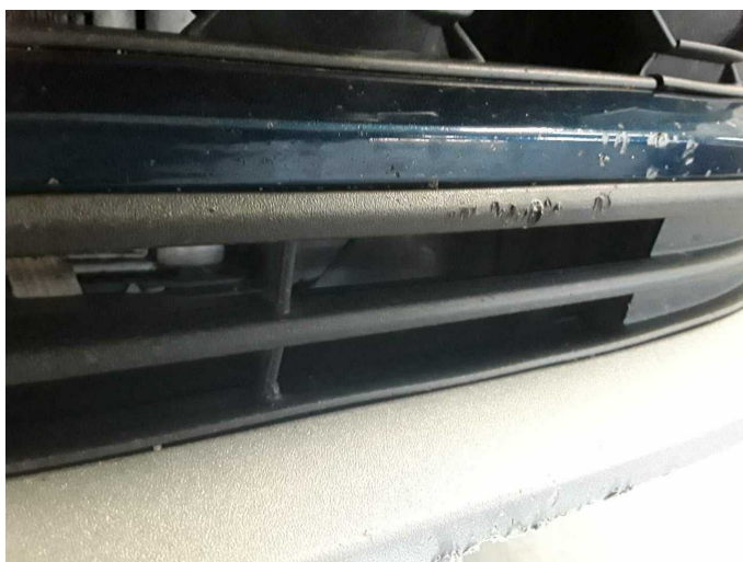
Damage 4: Front bumper: Cover bumper - front - Scratch(es) - Smart repair
