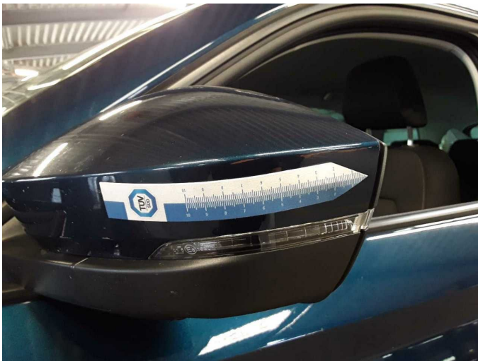
Wear and tear 10: Wing mirror - left side: Cap - Scratch(es) - Cover / polish
