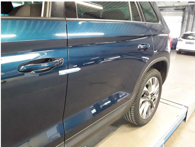
Wear and tear 7: Door - rear left side: Door - dent(s) - Smooth repair work
