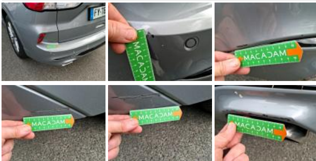
Bumper moulding R, Scratch(es), Paint
