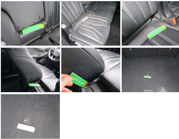
Interior trim, Missing, Replace
