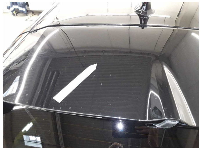
Damage 2: Boot lid / rear door: Rear spoiler - Scratch(es) - Smart repair value
