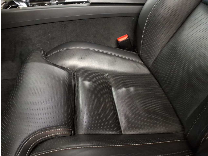
Damage 8: Seat - front: Seat cover - left side - Holes - Replace
