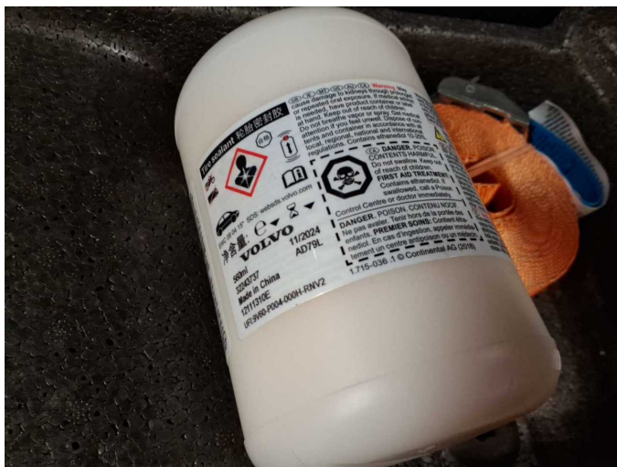
Damage 1: Equipment: Tirefit filler - Expired - Replace
