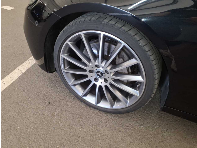
Damage 2: Wheel / tyres: Alloy rim - front left side - Scratch(es) - Loss in value
