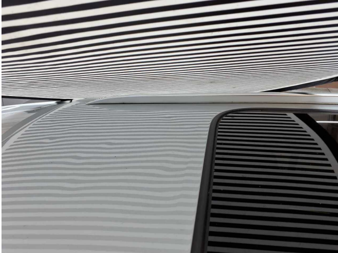
Damage 16: Roof: Roof - Deformed - Repair and paint
