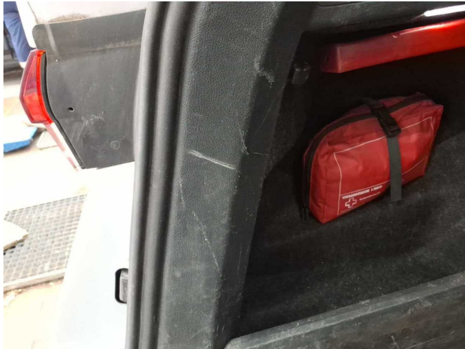
Damage 10: Interior: Interior - Scratch(es) - Loss in value
