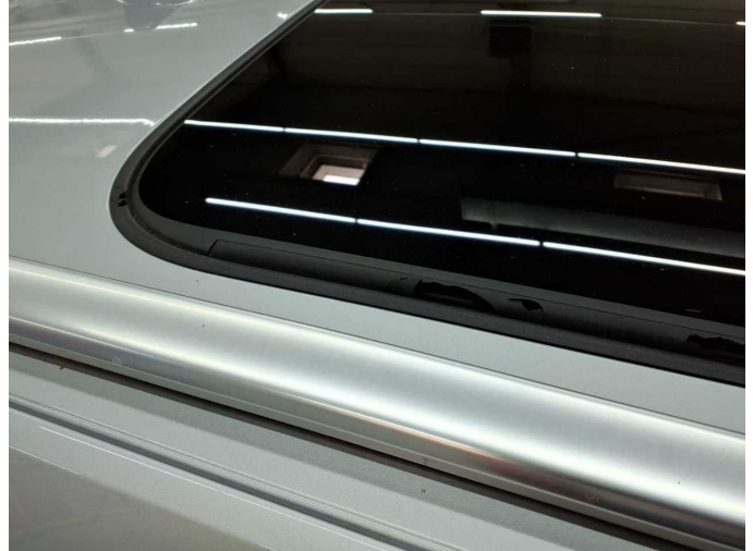
Damage 14: Roof: Roof hatch / sliding roof - seal - Broken / torn - Replace
