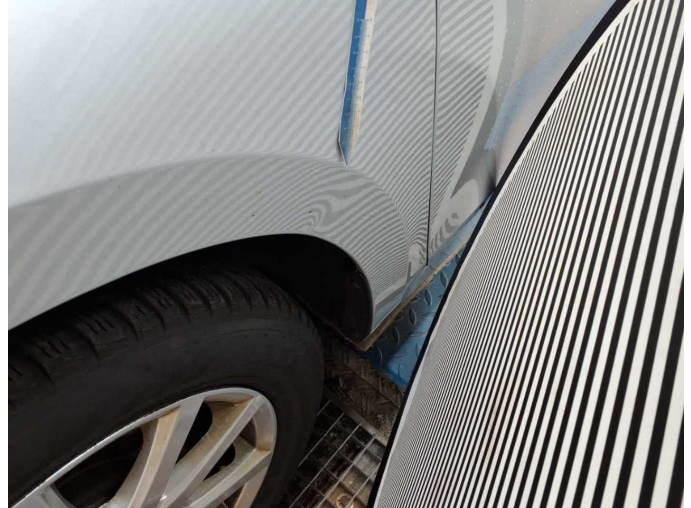
Damage 4: Mudguard - left side: Mudguard - left side - dent(s) - Smart repair
