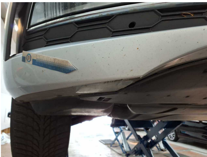
Damage 13: Front bumper: Front bumper - Scratch(es) - Paint
