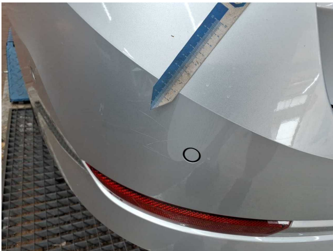
Damage 19: Rear bumper: Rear bumper - Dent / paintcoat damage - Replace
