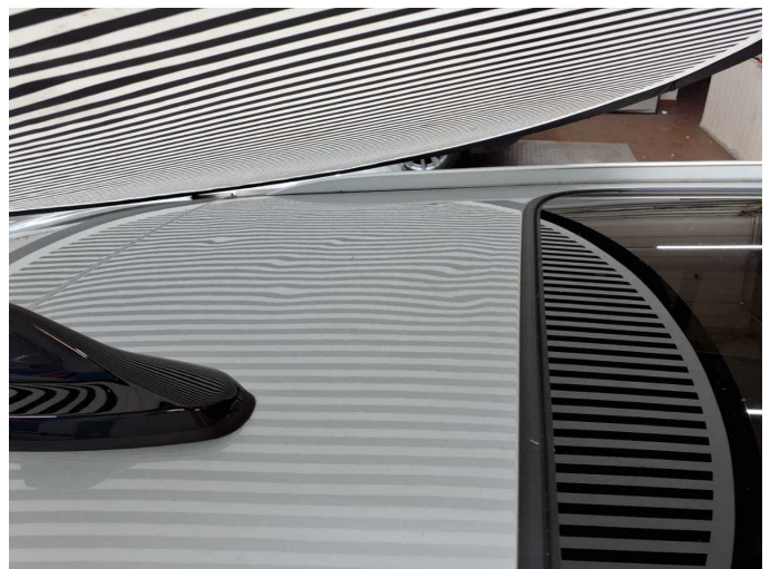
Damage 16: Roof: Roof - Deformed - Repair and paint
