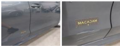
Sill trim R, Scratch(es), Repair and paint (complete)
