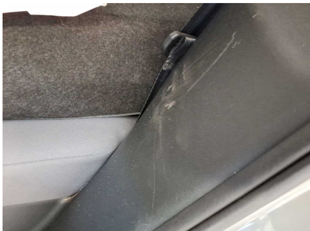
Damage #4: Side panel - rear left side: Interior trim - Scratched - Loss in value
