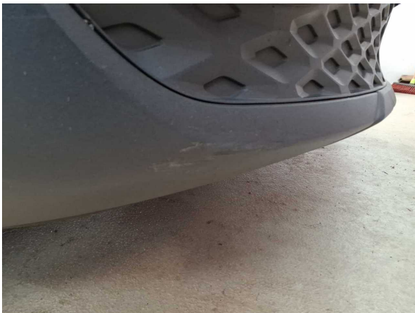
Damage #8: Front bumper: Spoiler - Scratched - Replace
