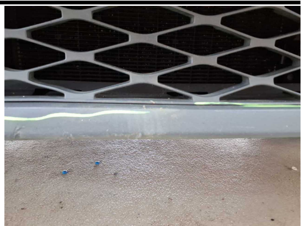
Damage #8: Front bumper: Spoiler - Scratched - Replace
