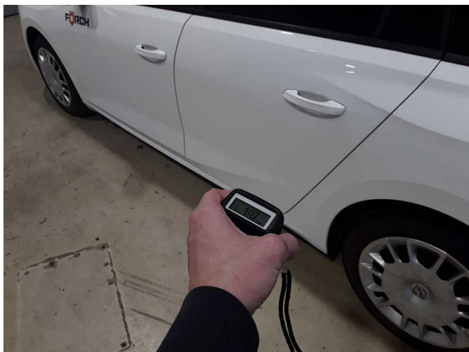
Repainting 2: Door - rear left side
