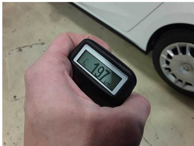
Repainting 2: Door - rear left side
