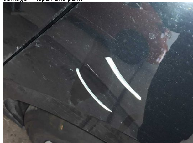
Damage #12: Side panel - rear left side: Side panel - Scratch... - Repair and paint
