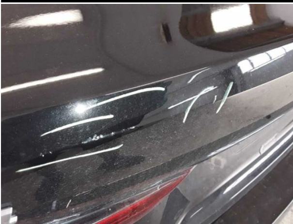
Damage #10: Boot lid / rear door: Boot lid - Scratched - Repair and paint
