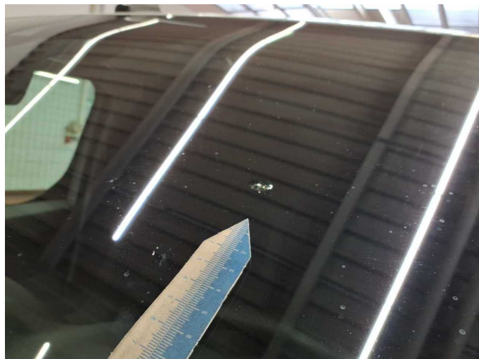
Damage 6: Vehicle glazing: Windscreen - Stone chips - Replace
