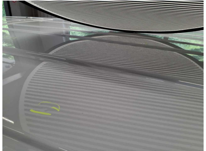
Damage 8: Body: Body - Damage by hail - Smooth repair work
