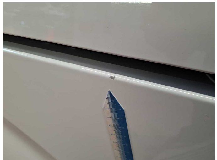
Damage 5: Side panel - rear right side: Side panel (+ Kratzer) - dent(s) - Smart repair
