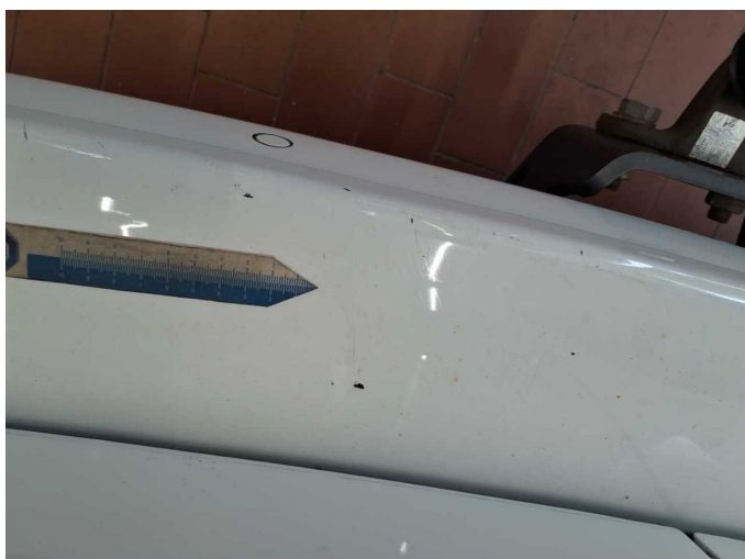
Damage 7: Rear bumper: Rear bumper - Scratch(es) - Paint
