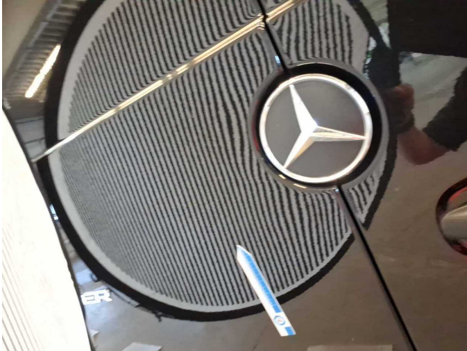
Damage 3: Boot lid / rear door: Rear door - left side - dent(s) - Smooth repair work
