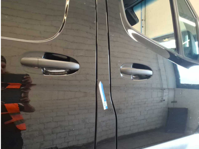
Damage 1: Body: B-pillar - right side - Scratch(es) - Smart repair
