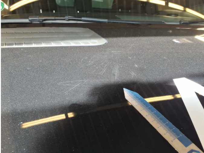
Damage 11: Bonnet: Bonnet - Scratch(es) - Paint
