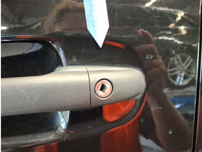
Damage 6: Door - front left side: Lock / Locking mechanism (Zylinder) - Broken / torn - Replace
