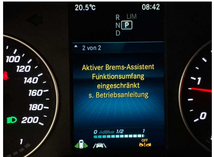
Damage 7: Electronic systems: Electronic systems (Assistensysteme) - Electrical fault - Perform diagnosis
