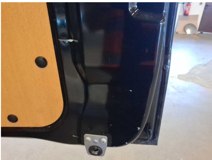
Wear and tear 2: Boot lid / rear door: Rear door - right side (Innenraum) - Scratched - No deduction
