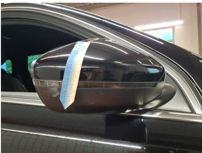
Damage 3: Indicator - front: Mirror - right side - Scratch(es) - Replace
