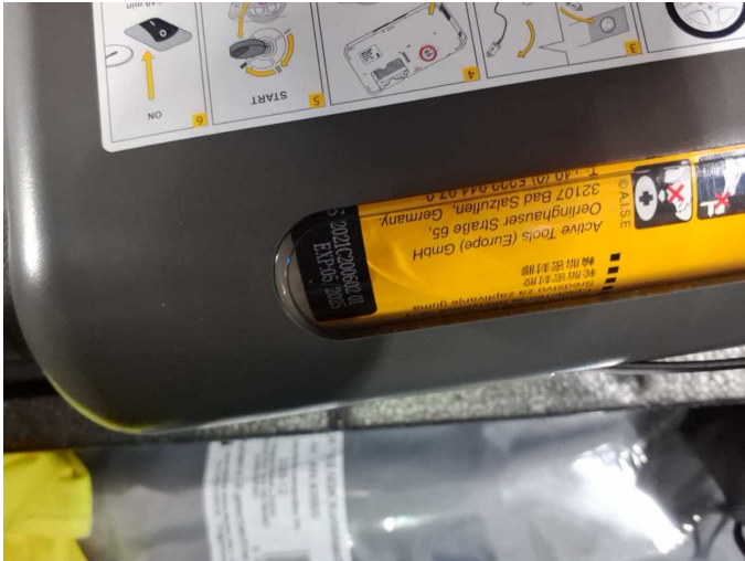
Damage 1: Equipment: Tirefit filler - Due - Replace
