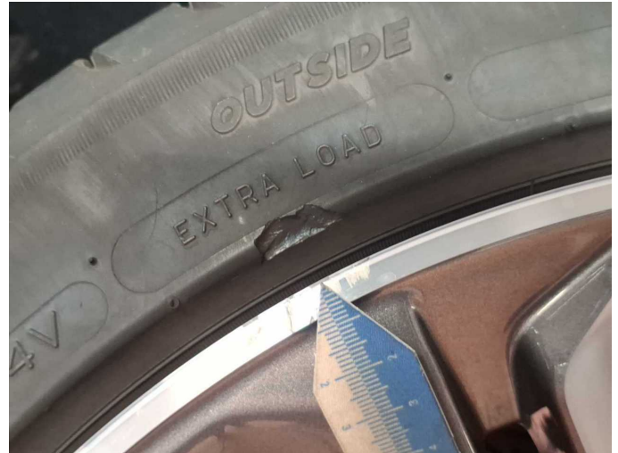
Damage 2: Wheel / tyres: Tyre - rear right side - Broken / torn - Replace
