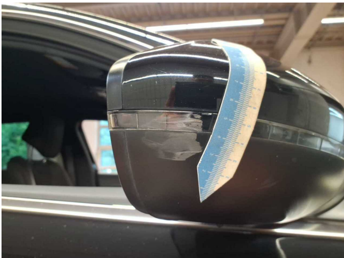
Damage 5: Wing mirror - right side: Mirror housing - Scratch(es) - Replace
