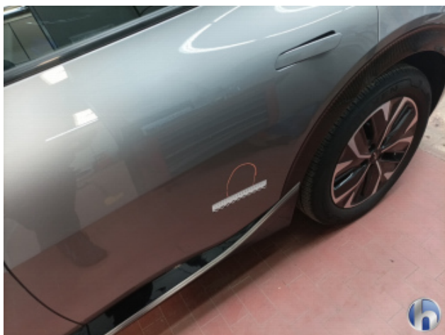
1. Tür Hinten - Links Delle - Sanft Instandsetzen
