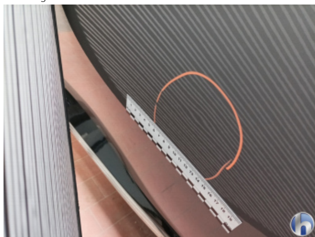
1. Tür Hinten - Links Delle - Sanft Instandsetzen
