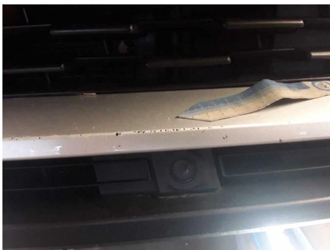
Damage 10: Front bumper: Spoiler - Scratched - Smart repair
