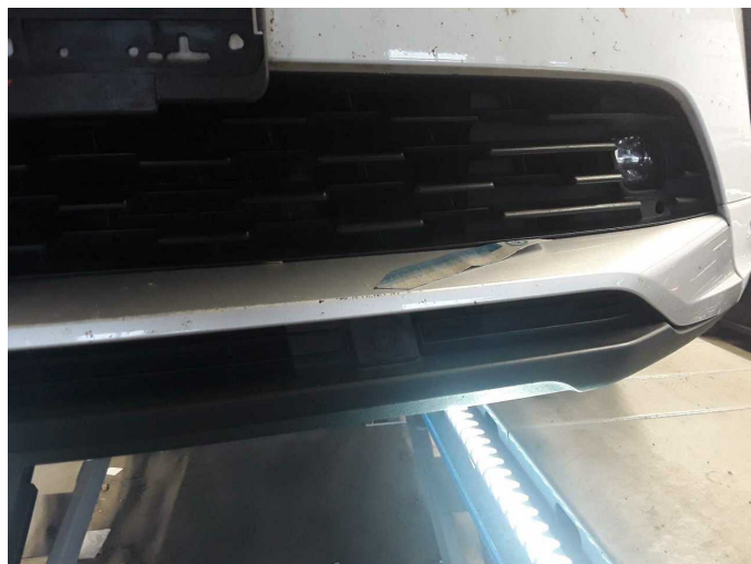
Damage 10: Front bumper: Spoiler - Scratched - Smart repair
