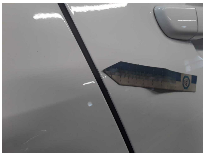
Damage 5: Door - rear right side: Door - Scratched - Smart repair
