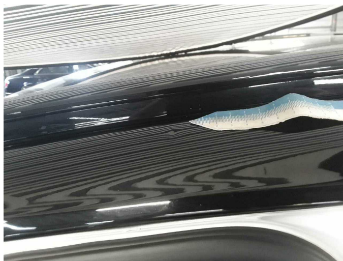
Damage 6: Roof: Roof rail - left side - dent(s) - Smooth repair work
