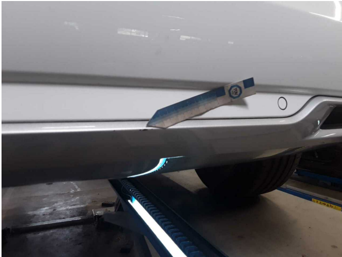
Damage 8: Rear bumper: Spoiler - Scratched - Smart repair
