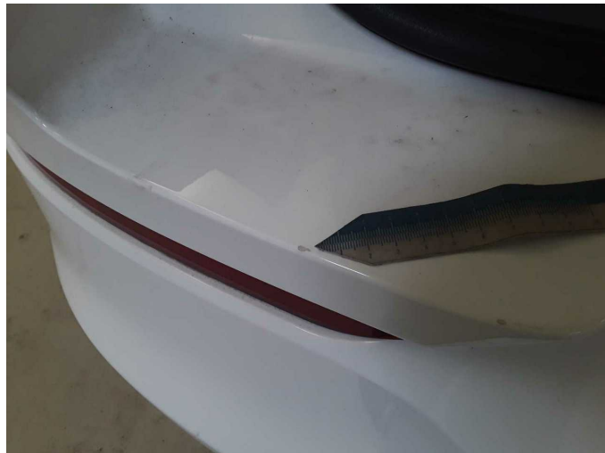
Damage 3: Rear bumper: Rear bumper - Scratched - Cover / polish
