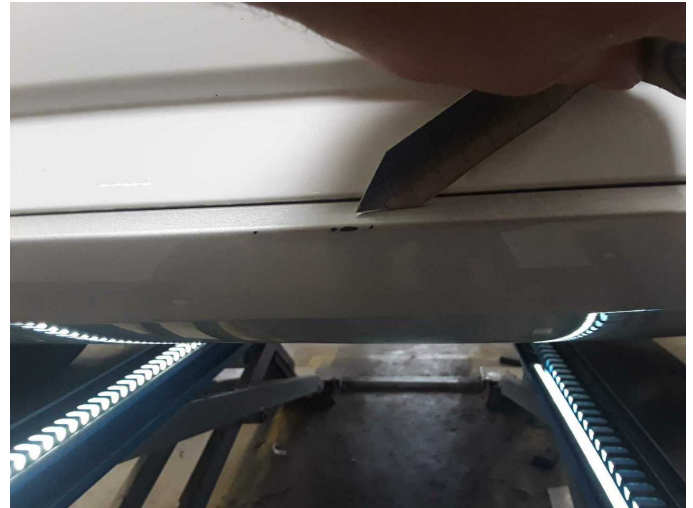
Damage 8: Rear bumper: Spoiler - Scratched - Smart repair
