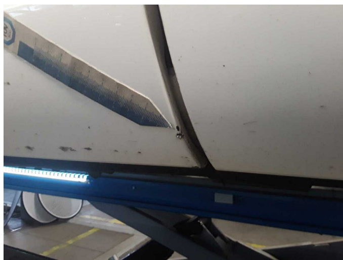
Damage 4: Trim / covers: Door trim - front left side - Scratched - Smart repair
