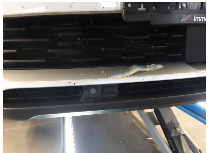
Damage 10: Front bumper: Spoiler - Scratched - Smart repair
