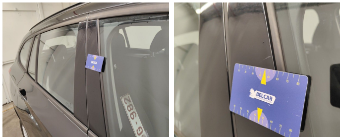
Door Front Right / Trim / Replace-scratch
