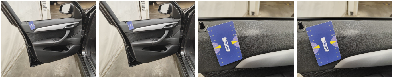
Front Left Door Interior Coating // Replace Completely-scratch
