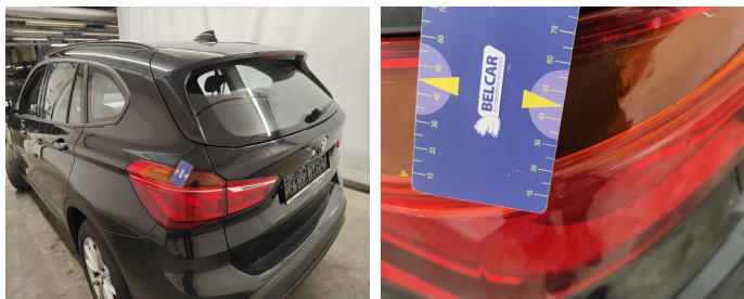
Light / Rear left / Replace-scratch
