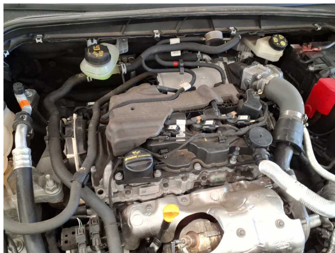
Missing part 1: Engine: Engine cover - Missing - Replace
