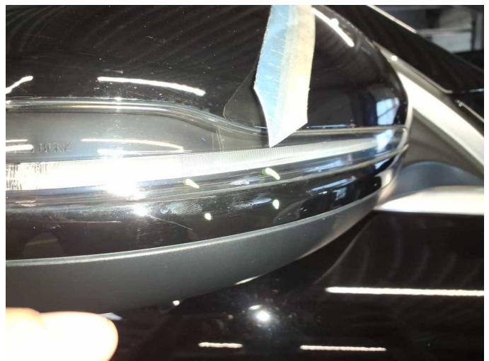
Damage 7: Indicator - front: Mirror - right side - Broken / torn - Replace
