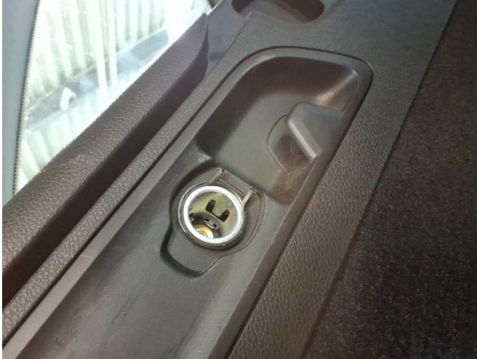
Damage 1: Electrical system: Power socket - Damaged - Replace
