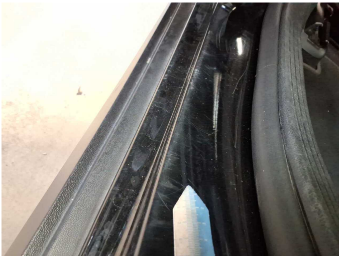
Damage 4: Sill - left side: Sill - Scratch(es) - Smart repair
