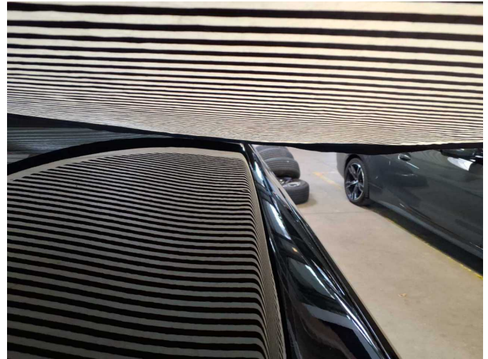
Damage 13: Bonnet: Bonnet - dent(s) - Paint
