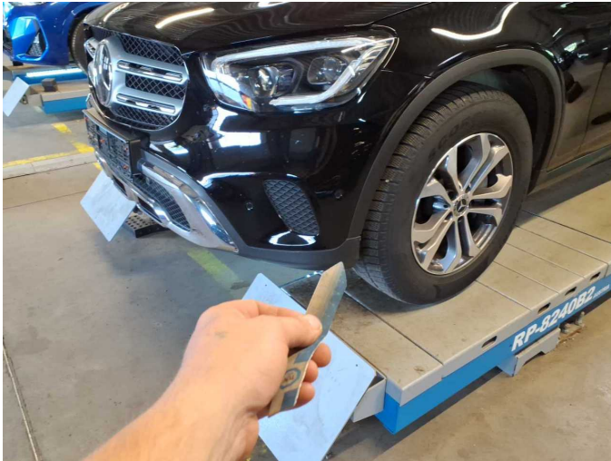
Damage 8: Front bumper: Spoiler - Scratched - Loss in value
