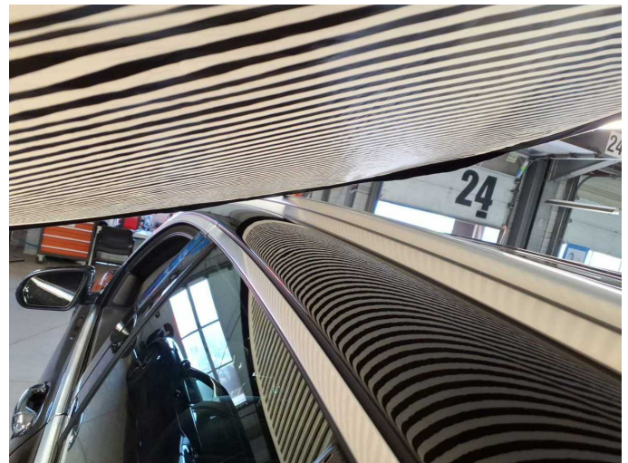
Wear and tear 3: Roof: Roof rail - left side - dent(s) - No deduction
