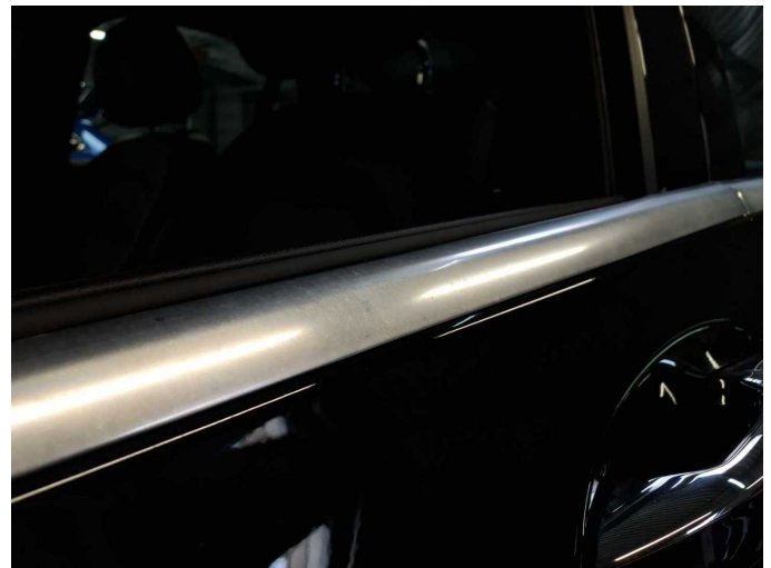
Damage 10: Body: Body (Chromleisten und Dachreling) - Paint defect - Loss in value
