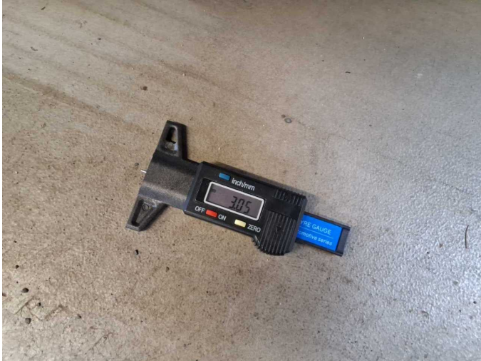
Damage 11: Wheel / tyres: Tyres - complete set (Winterreifen) - Worn - Replace
