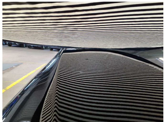
Damage 13: Bonnet: Bonnet - dent(s) - Paint
