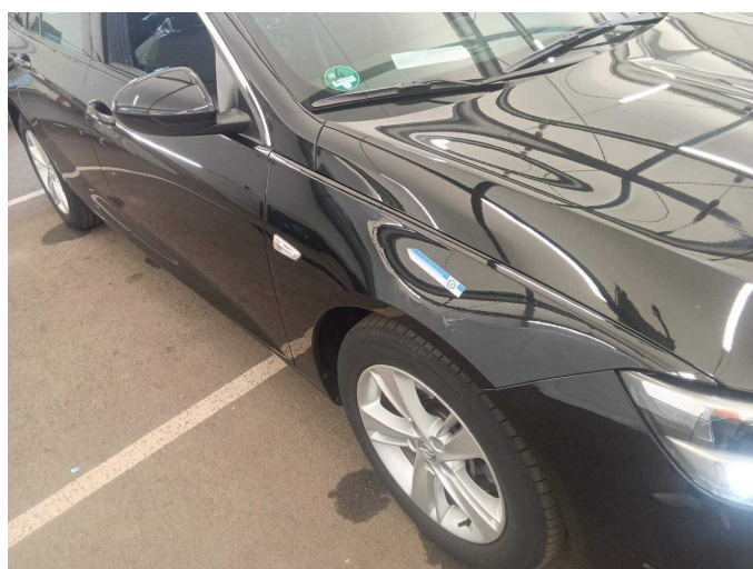
Damage 5: Mudguard - right side: Mudguard - right side - dent(s) - Smooth repair work
