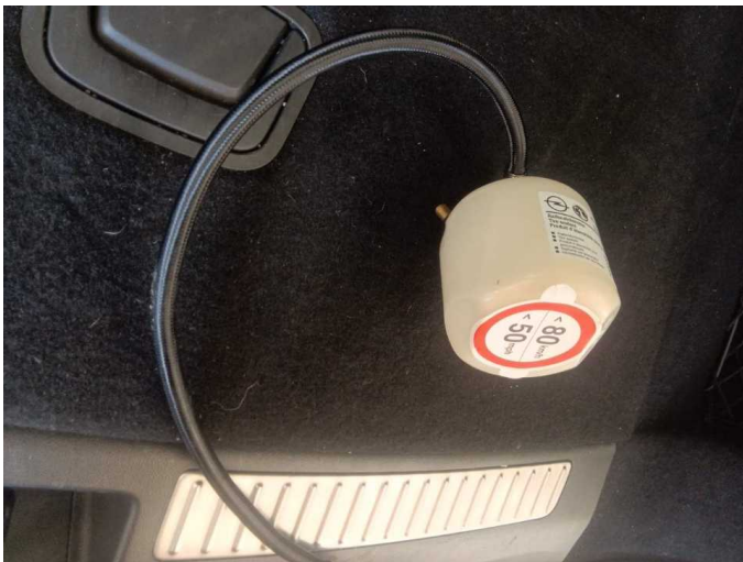
Damage 1: Equipment: Tirefit filler - Empty - Replace
