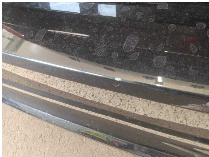
Damage 3: Rear bumper: Rear bumper - Scratch(es) - Paint
