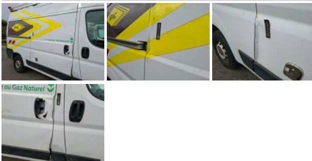
Outer door handle RR, Broken, Replace
