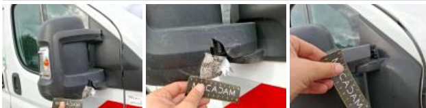
Side panel moulding R, Broken, Replace
