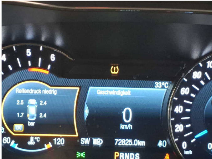
Damage 2: Instrument panel: Indicator light (Reifendruck Kontrollleuchte) - on - Perform diagnosis
