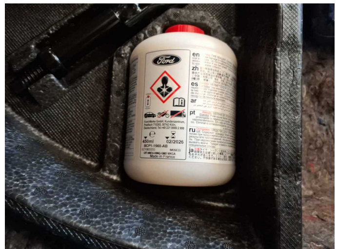
Damage 1: Equipment: Tirefit filler - Expired - Replace
