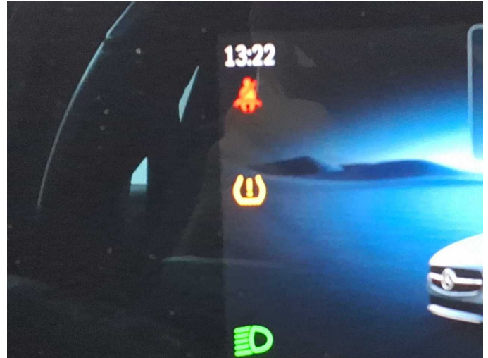
Damage 2: Instrument panel: Indicator light (Reifendruckkontrollsystem) - on - Perform diagnosis
