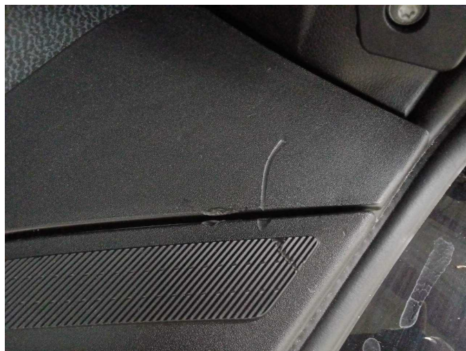
Damage 2: Trim / covers: Boot sill cover - Scratch(es) - Replace
