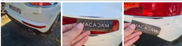
Fog light RR, Broken, Replace
