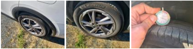
Tyre RR, Out of tolerance, Replace
