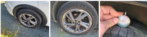
Tyre FR, Out of tolerance, Replace
