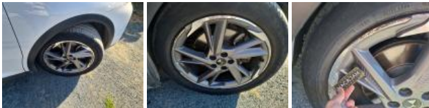
Tyre FL, Out of tolerance, Replace
