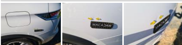
Door RL, Dent(s), Repair and paint (complete)
