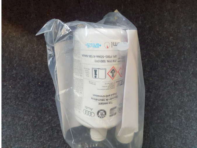
Damage 1: Equipment: Tirefit filler - Expired - Replace
