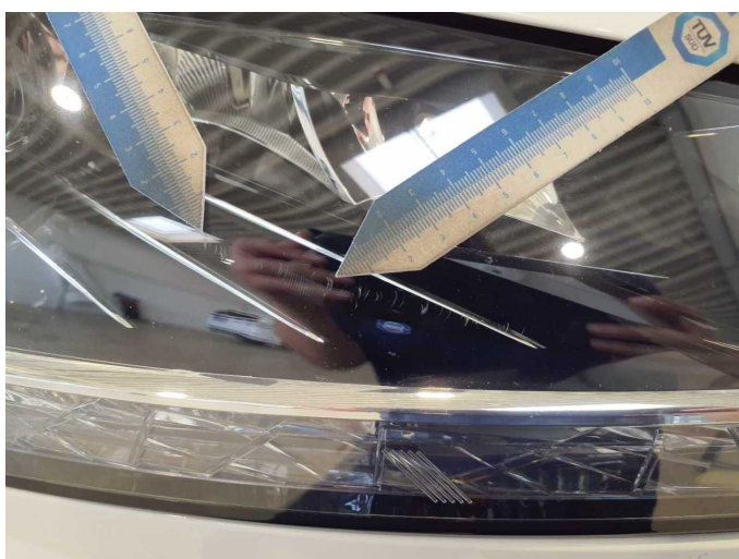
Damage 7: Headlight: Headlight - right side - Scratch(es) - Replace
