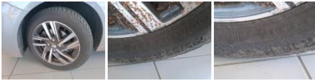
Tyre RL, Out of tolerance, Replace
