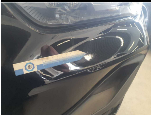
Damage #4: Front bumper: Front bumper - Stone chips - Smart repair
