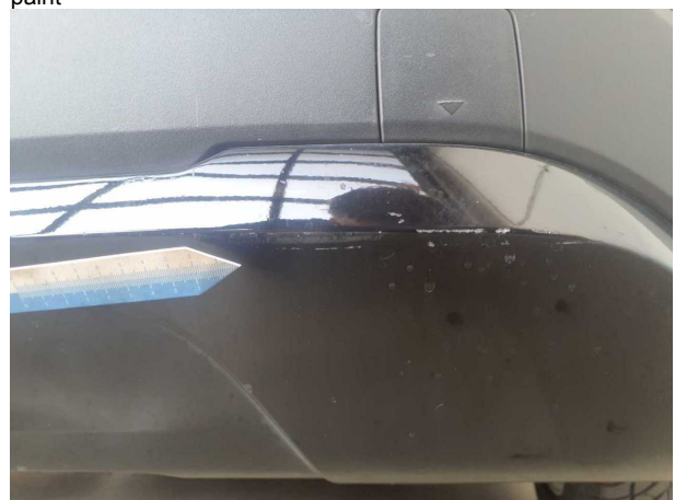
Damage #5: Rear bumper: Spoiler - Scratch(es) - Repair and paint
