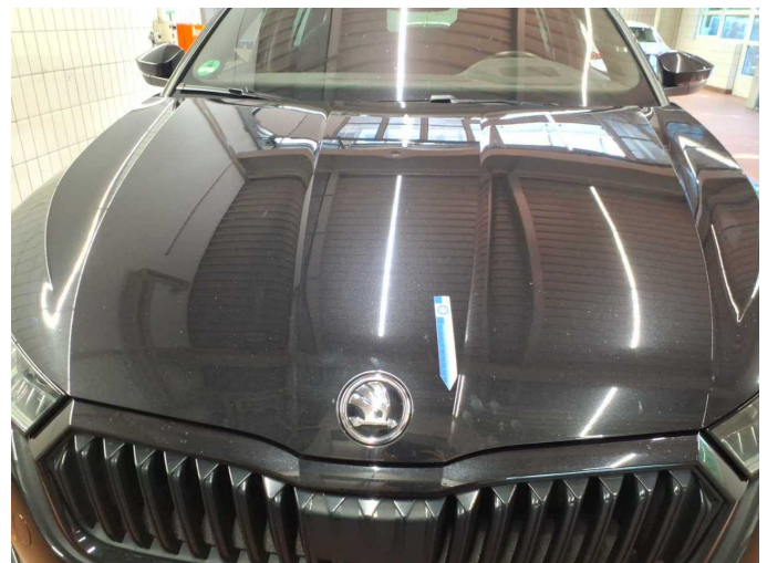
Damage 2: Bonnet: Bonnet - dent(s) - Smooth repair work
