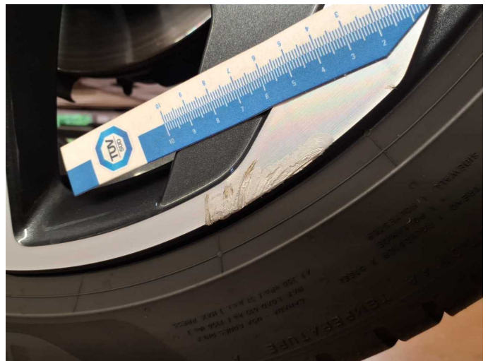
Damage 4: Wheel / tyres: Alloy rim - front right side - Scratch(es) - Replace
