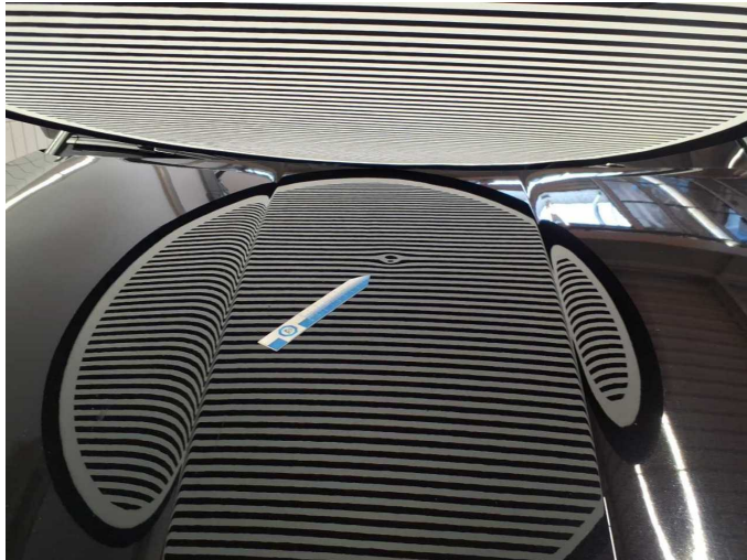
Damage 2: Bonnet: Bonnet - dent(s) - Smooth repair work
