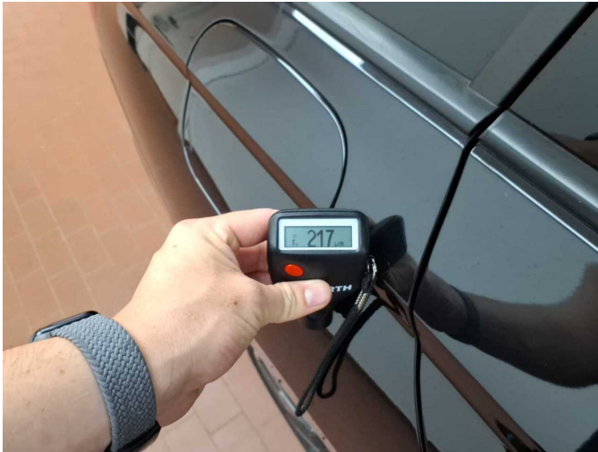
Repainting 2: Side panel - rear right side
