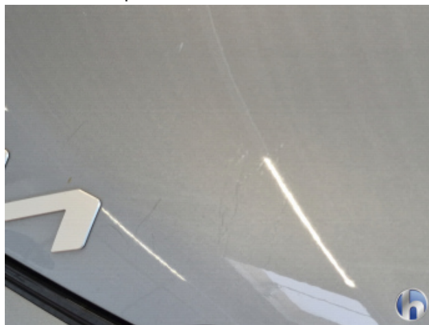
2. Motorhaube Kratzer - Smart Repair
