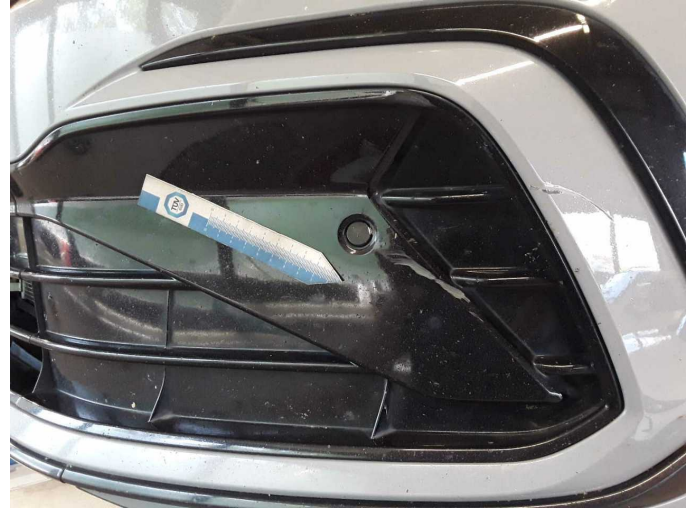
Damage 3: Front bumper: Parking sensors - left side - Damaged - Replace
