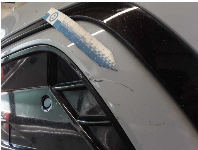
Damage 6: Front bumper: Front bumper - Scratched - Paint
