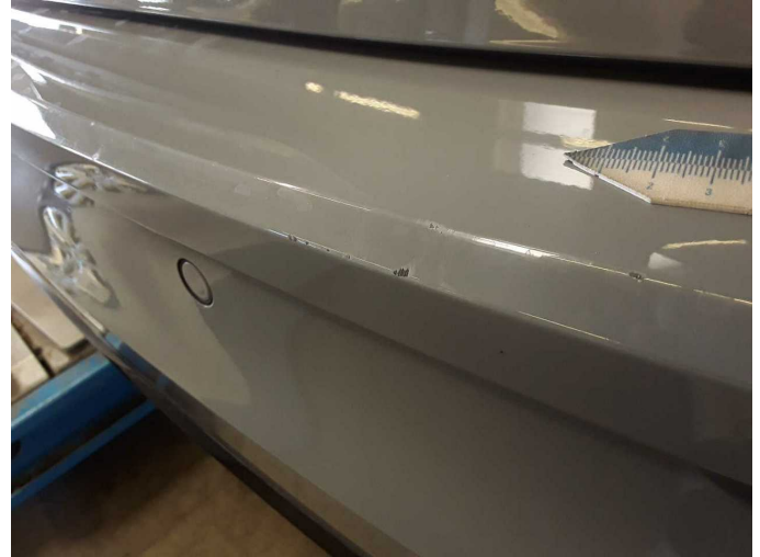
Damage 5: Rear bumper: Rear bumper - Scratch(es) - Paint
