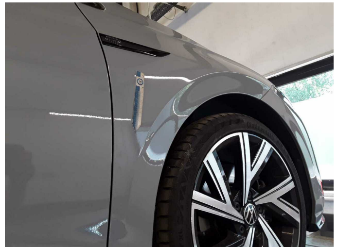
Damage 4: Mudguard - right side: Mudguard - right side - Deformed - Repair and paint
