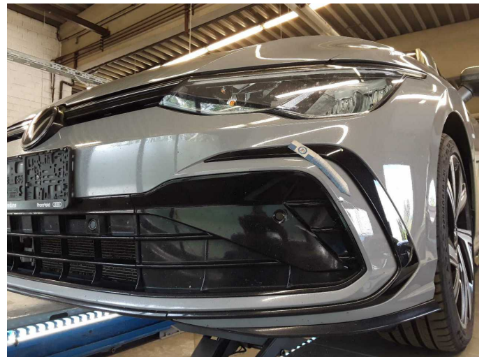
Damage 6: Front bumper: Front bumper - Scratched - Paint
