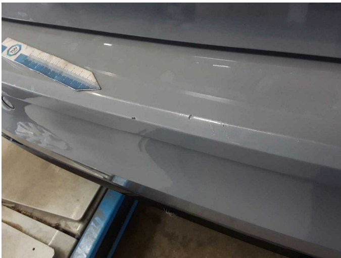
Damage 5: Rear bumper: Rear bumper - Scratch(es) - Paint
