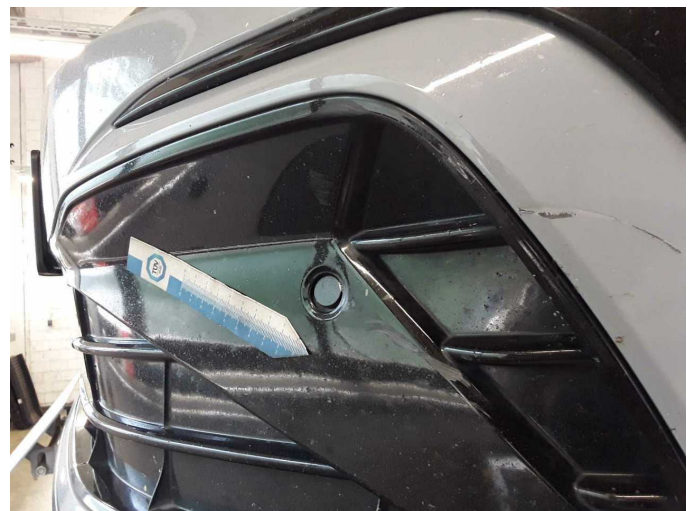
Damage 6: Front bumper: Front bumper - Scratched - Paint
