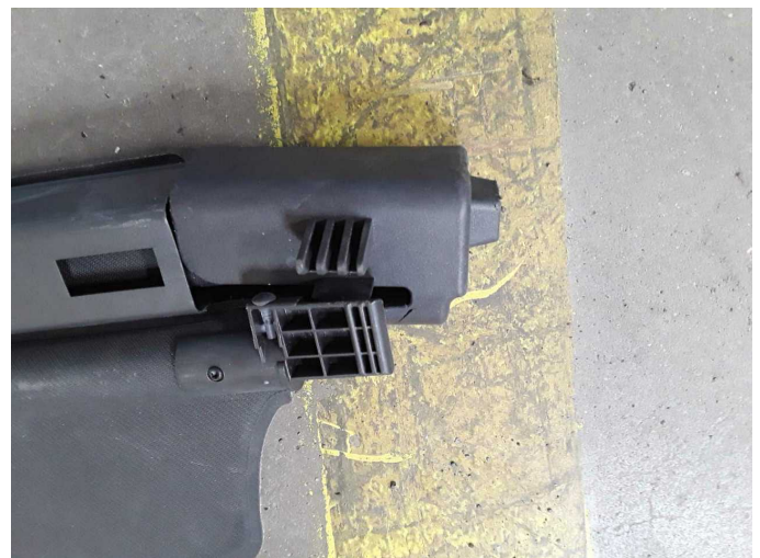
Damage 3: Interior: Boot cover / roller cover - Damaged - Replace
