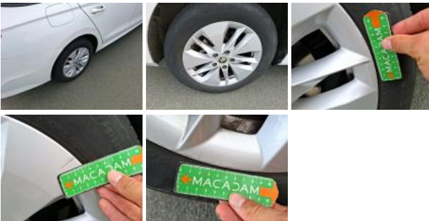
Tyre RL, Out of tolerance, Replace
