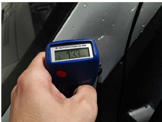
Dachholm links: 133 µm
