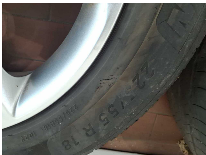
Damage 15: 2nd wheel set: 2 tyres - Damaged - Replace
