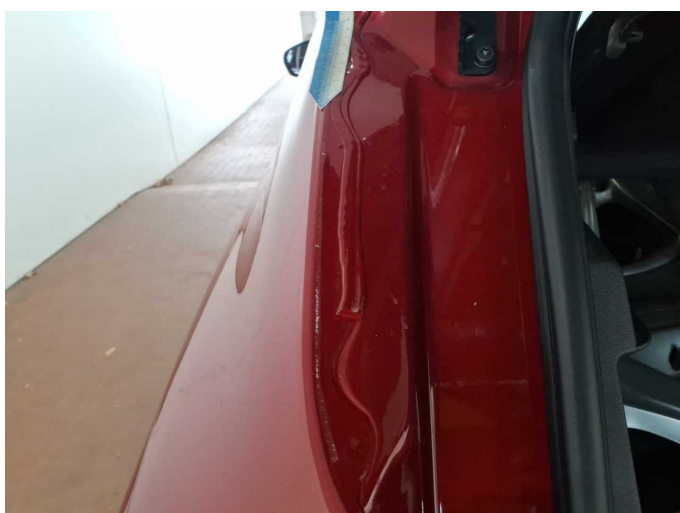
Damage 13: Side panel - rear left side: Side panel - Scratch(es) - Smart repair
