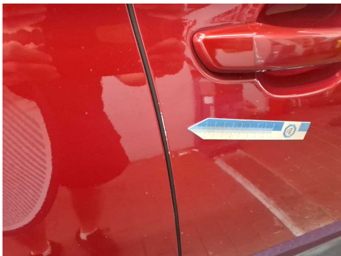
Damage 9: Door - front right side: Door edge - Scratch(es) - Smart repair
