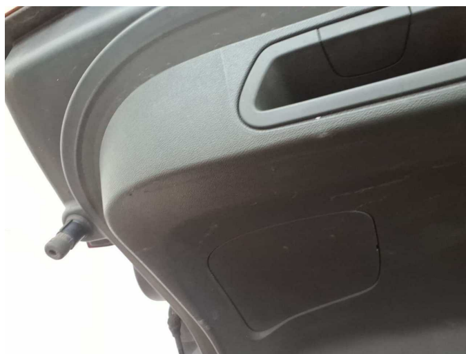
Damage 4: Trim / covers: Boot lid - interior trim - Scratch(es) - Loss in value
