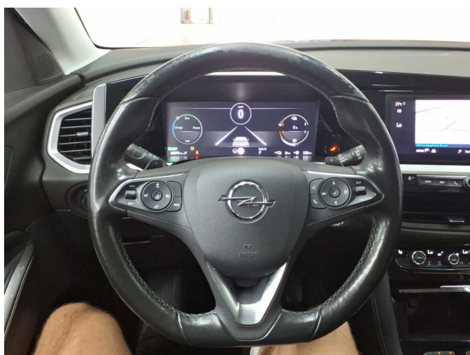
Damage 8: Steering system: Steering wheel - Abrasion - Loss in value
