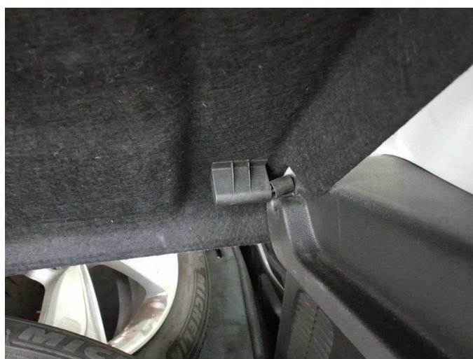
Damage 14: Interior: Rear shelf (Halter gerissen) - Damaged - Replace
