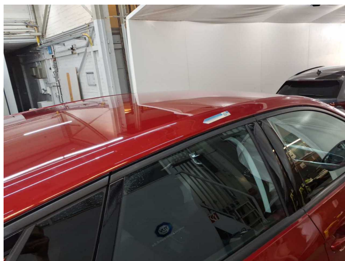
Damage 11: Roof: Roof rail - right side - dent(s) - Smart repair
