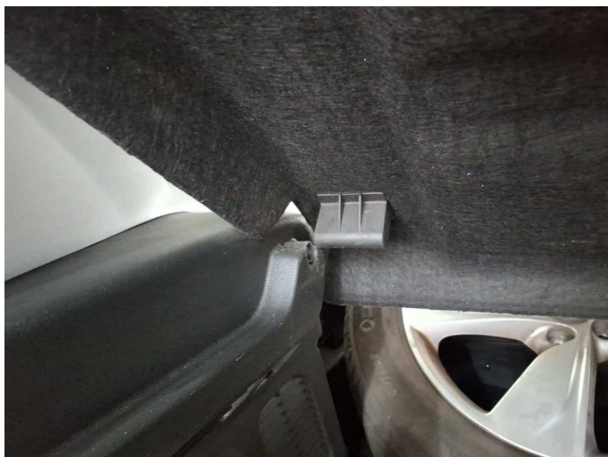
Damage 14: Interior: Rear shelf (Halter gerissen) - Damaged - Replace
