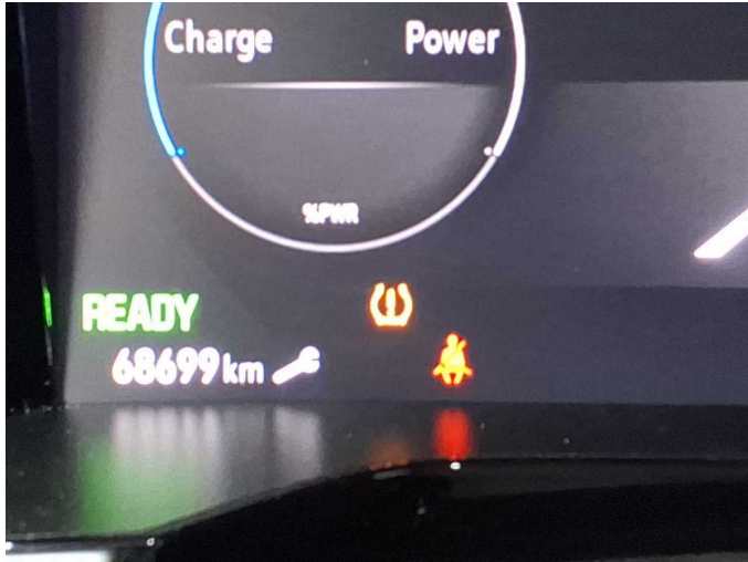
Damage 5: Instrument panel: Indicator light (Reifendruckkontrollsystem) - on - Perform diagnosis
