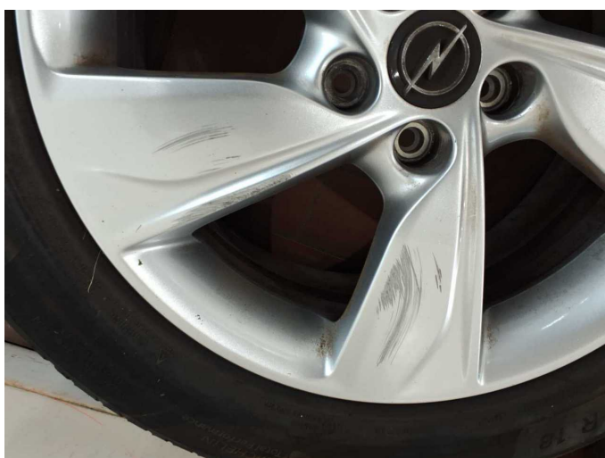
Damage 18: 2nd wheel set: 3 alloy rims - Scratch(es) - Loss in value
