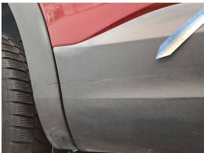
Damage 16: Side panel - rear right side: Wheel arch (+ Zierleiste Tür) - Scratched - Replace
