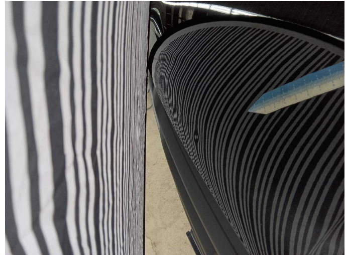
Damage 2: Bonnet: Bonnet - dent(s) - Smooth repair work
