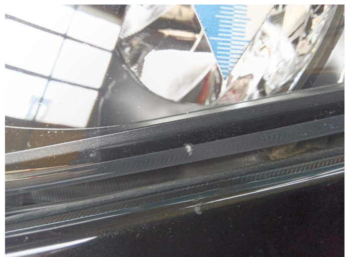
Damage 4: Headlight: Headlight - left side - Stone chips - Replace
