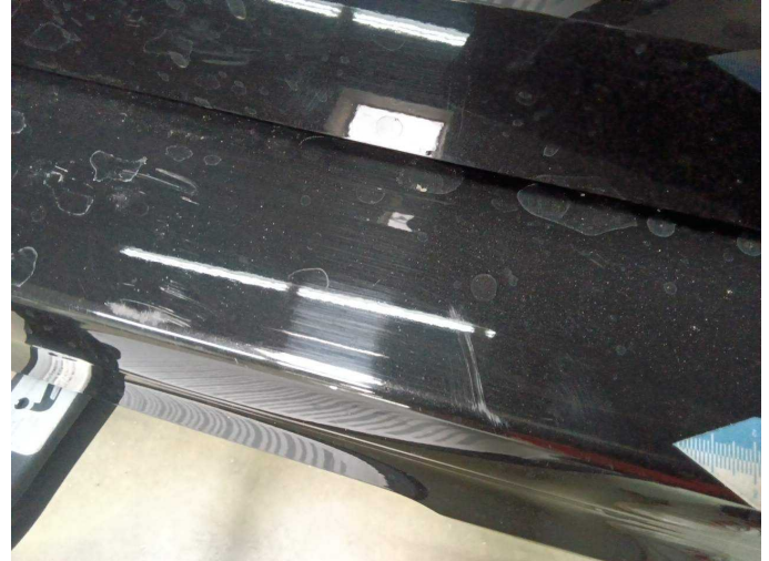
Damage 5: Rear bumper: Rear bumper - Scratch(es) - Paint
