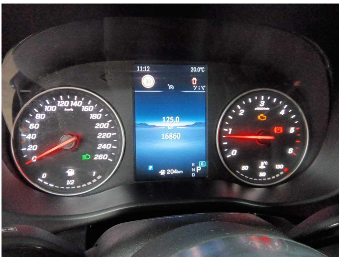
Damage 3: Instrument panel: Indicator light (Motorkontolleuchte) - on - Perform diagnosis
