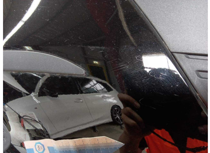
Damage 7: Front bumper: Front bumper - Scratch(es) - Paint
