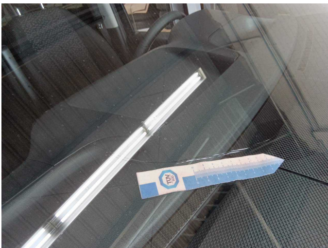
Damage 8: Vehicle glazing: Windscreen - Broken / torn - repair according to calculation
