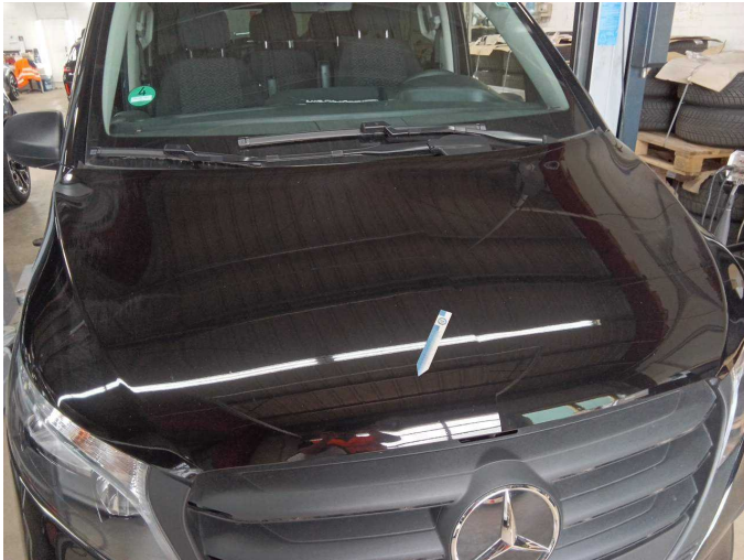
Damage 2: Bonnet: Bonnet - dent(s) - Smooth repair work
